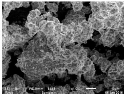
**Figure 1: Porous microstructure of loess loam**
