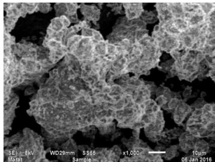
**Figure 1: Porous microstructure of loess loam**
