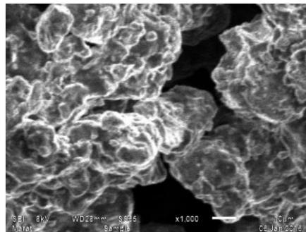
**Figure 2: Microstructure of organo-mineral conglomerate mixture with oil sludge.**
